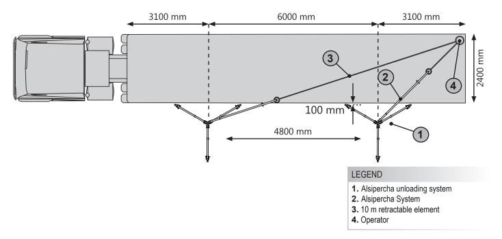
Any operator unloading a truck with 12 m platform, must use:
