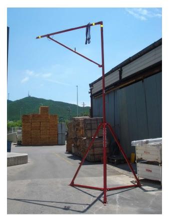
**IMPORTANT NOTE:** It is very important to assemble the ALSIPERCHA TRIPOD on sufficiently compact ground so that it can be securely anchored. There are various ground/sole plate/foundation options:
