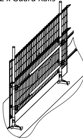
Increase fixings loads by 2kN compared to High Barrier (or Std Barrier + Make-up Barrier) to maintain wind loads as shown in respective TD sheet.
