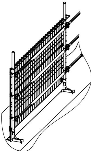
Increase fixings loads by 3kN compared to High Barrier (or Std Barrier + Make-up Barrier) to maintain wind loads as shown in respective TD sheet.
