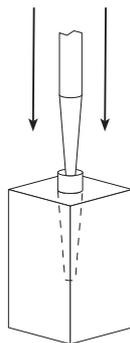
2.- Use the leveller to make sure that the tube is vertical and does not rise up. The column is strengthened by the housing tube.
