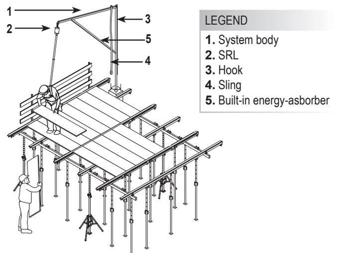
Alsipercha is CE certified in accordance with the DIN EN 795 type B (Notified Body 0158, DEKRA EXAM)
