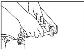
Detail of the installation of the retractable device with the fall arrest system. It is important to close the clasp properly.
