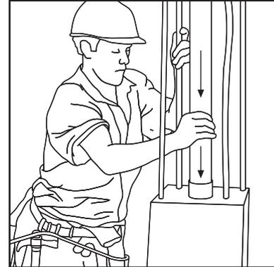
2.- 36 hours after pouring the column concrete, the Alsipercha can be used to: install boards, handrails, risers,...
