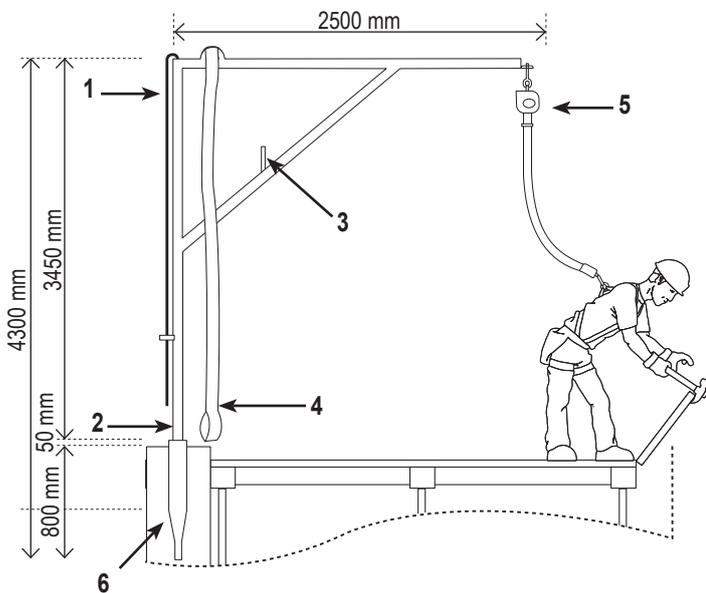
Technical details for arranging the housing tube.
