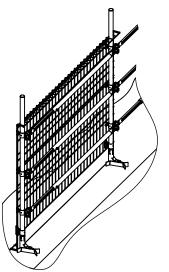
Increase fixings loads by 3kN compared to High Barrier (or Std Barrier + Make-up Barrier) to maintain wind loadsas shown in respective TD sheet. Alt. 2
