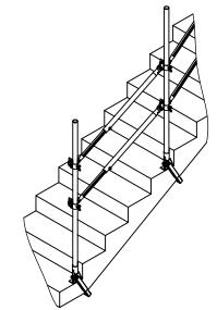
Fixing and wind loads are equal to non raised standard barrier as shown in respective TD sheet.
