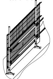
Increase fixings loads by 2kN compared to High Barrier (or Std Barrier + Make-up Barrier) to maintain wind loads as shown in respective TD sheet.
