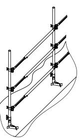
Fixing and wind loads are equal to non raised standard barrier as shown in respective TD sheet.
