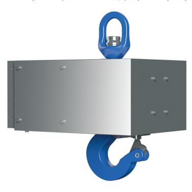
Made of ST 37-2 Steel Galvanized surface treatment Compatible with the complete range of automatic hooks (except evo2). Approximate weight of 17 kg / 37.47 lb Dimensions: 285 x 195 x 425 mm / 11.22 x 7.67 x 16.73 in
