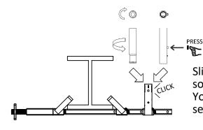
Slide the V-Post into the post socket on the HD Flange Clamp. You will hear a click when it is secured.
