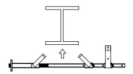
Loosen off wing nut to allow the HD Flange Clamp to fit over the I-Beam.
