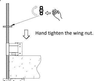
Use a hammer to tighten the wing nut **HALF A REVOLUTION**past hand tight and secure the HD Clamp to the concrete slab.
